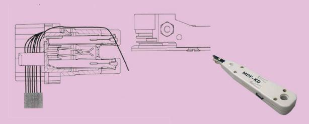
The wires are positioned in the cable grips with an overlength of approximately 100 mm and then terminated by using the insertion tool.
